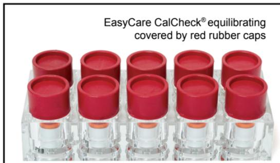
**CHECKING THE CALIBRATION OF YOUR SENSORS:** The EasyCare CalCheck® used to verify calibration of your Rapid RH® 5.0 Smart Sensors. The ASTM F2170 test standard calls for checking sensor (probe) calibration 30 days before use.
