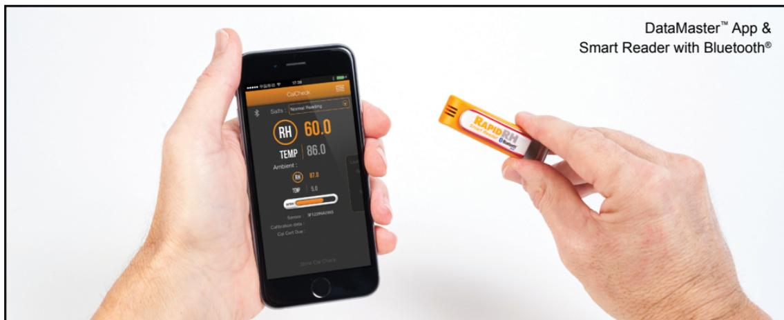
If using the Smart Reader with the Rapid RH® DataMaster™ app, as mentioned earlier, sensors' readings will be stored in the app and can be uploaded to the [f2170reports.com](http://f2170reports.com) website.
