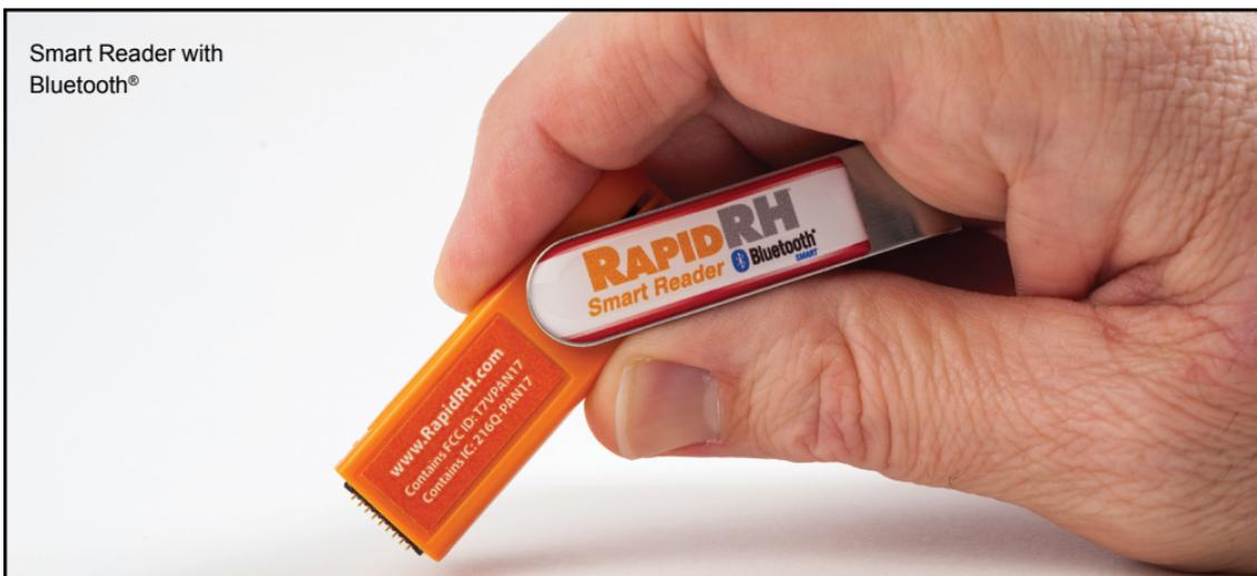
The Rapid RH® Smart Sensor's patented design equilibrates (acclimates) faster than any other concrete relative humidity sensing device. Project scheduling decisions regarding the slab can usually be made one hour after installation. Just remember to follow the ASTM F2170 procedures pertaining to minimum equilibration time for correct and required reporting of the test results.
