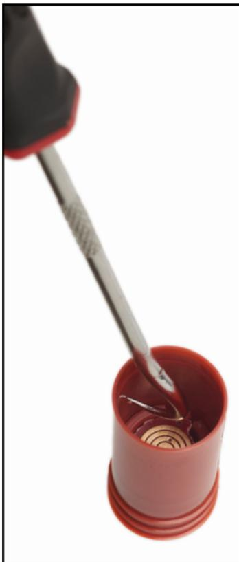
the tool counterclockwise while pulling up. If you are going to be doing future testing of this hole, make sure you put a protective cap on the sleeve. When ready to obtain additional readings, you can just reverse the above removal process to reinstall the Smart Sensor into the Base Sleeve.
