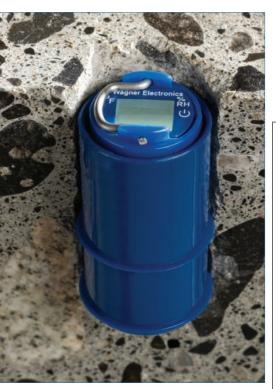
The Wagner Electronics Rapid RH<sup>™</sup> Smart Sensor is ¾" in diameter, and measures both temperature and relative humidity within the slab.
