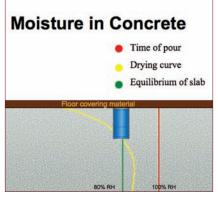
Once a floor covering is installed, the relative humidity equilibrates throughout the slab (green line). Taking readings at 40% depth (slab on grade) prior to installation of a floor covering tells us what the slab will eventually equilibrate to after the floor covering has been placed (intersection of yellow and green line).
