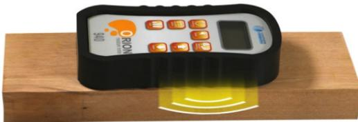
The 2.0-inch (50mm) wide by 2.5-inch (63mm) long by either .25-inch (6mm) or .75-inch (19mm) thick sensor field of your Orion® moisture meter closely approximates the full-thickness cross-section method used when performing the ASTM D4442-16 oven-dry lab method. This ASTM standard (and its international counterparts) is the standard to which all moisture meters for wood are compared for accuracy.
