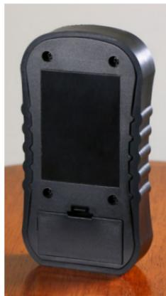
*\*Although not recommended, you may wish to use the meter without the protective rubber boot. If you choose to do so, make sure you recalibrate your meter on the On-Demand Calibrator with the boot off.*
