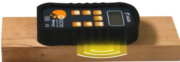
The 2.0-inch (50mm) wide by 2.5-inch (63mm) long by either .25-inch (6mm) or .75-inch (19mm) thick sensor field of your Orion® moisture meter closely approximates the full-thickness cross-section method used when performing the ASTM D4442-16 oven-dry lab
