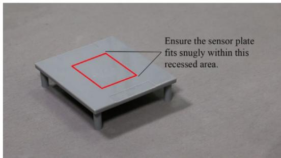
1. Place the Calibrator on its legs on a non-metallic surface.
