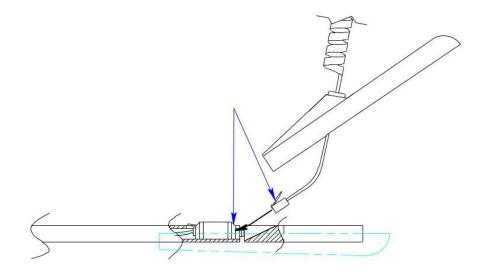
**Step 6**. Carefully stow service loop and reassemble handle. See Step 1 for screw locations.
