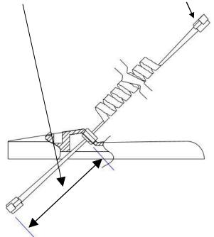
**Step 5**. Connect Replacement cord to coupler. Ensure latch clicks into detent.
