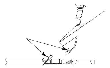
**Step 3**. Loosen (2) inside extrusion screws, then remove (2) outside hinge dock screws. Gently pull the Probe Head and its attached cable from the extrusion.
