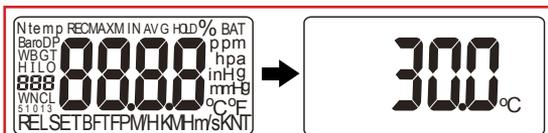
The meter displays full segments in 1 second and then TEMP icon with reading appears on the LCD with a beep sound. To turn off the meter, press **POWER** button for more than 2 seconds.
