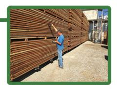
The Model L722 Stack Probe Sensor – coupled with the L622 Digital Recording Moisture Meter – makes it easy to reach deep into stickered units of lumber and take accurate moisture readings without the danger of broken pins. Ruggedly-built, the L722 can take accurate in-kiln readings, even when temperatures reach 200° F (93° C) or more, or take readings of lumber removed from the kiln and stored prior to planing.
